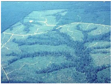
An SMZ, a minimum of 50 feet wide, should be left along both sides of all perennial and intermittent streams.
