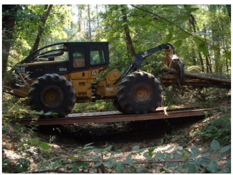
Stream crossings should be kept to a minimum, designed to accommodate the intended traffic level, and installed properly to minimize disturbance to the stream bank and channel.
